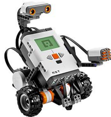
Figure 2. A LEGO® NXT Brick with Ultrasonic Sensor
